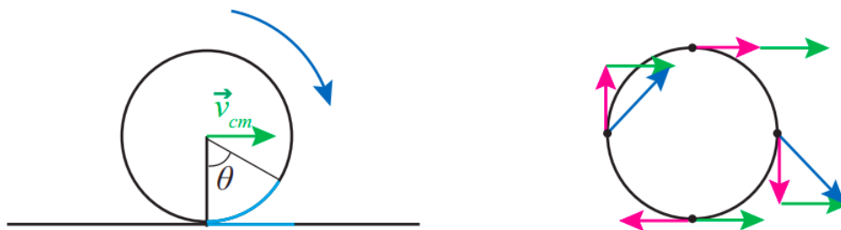
Figure 9.6.1: Left: illustrating the rolling without slipping condition. The cyan line on the surface has the same length as the cyan-colored arc, and will be the distance traveled by the disk when it has turned through an angle \theta . Right: velocities for four points on the edge of the disk. The pink arrows are the velocities in the center of mass frame. In the Earth reference frame, the velocity of the center of mass, \vec{v}_{cm} , in green, has to be added to each of them. The resultant is shown in blue for two of them.
