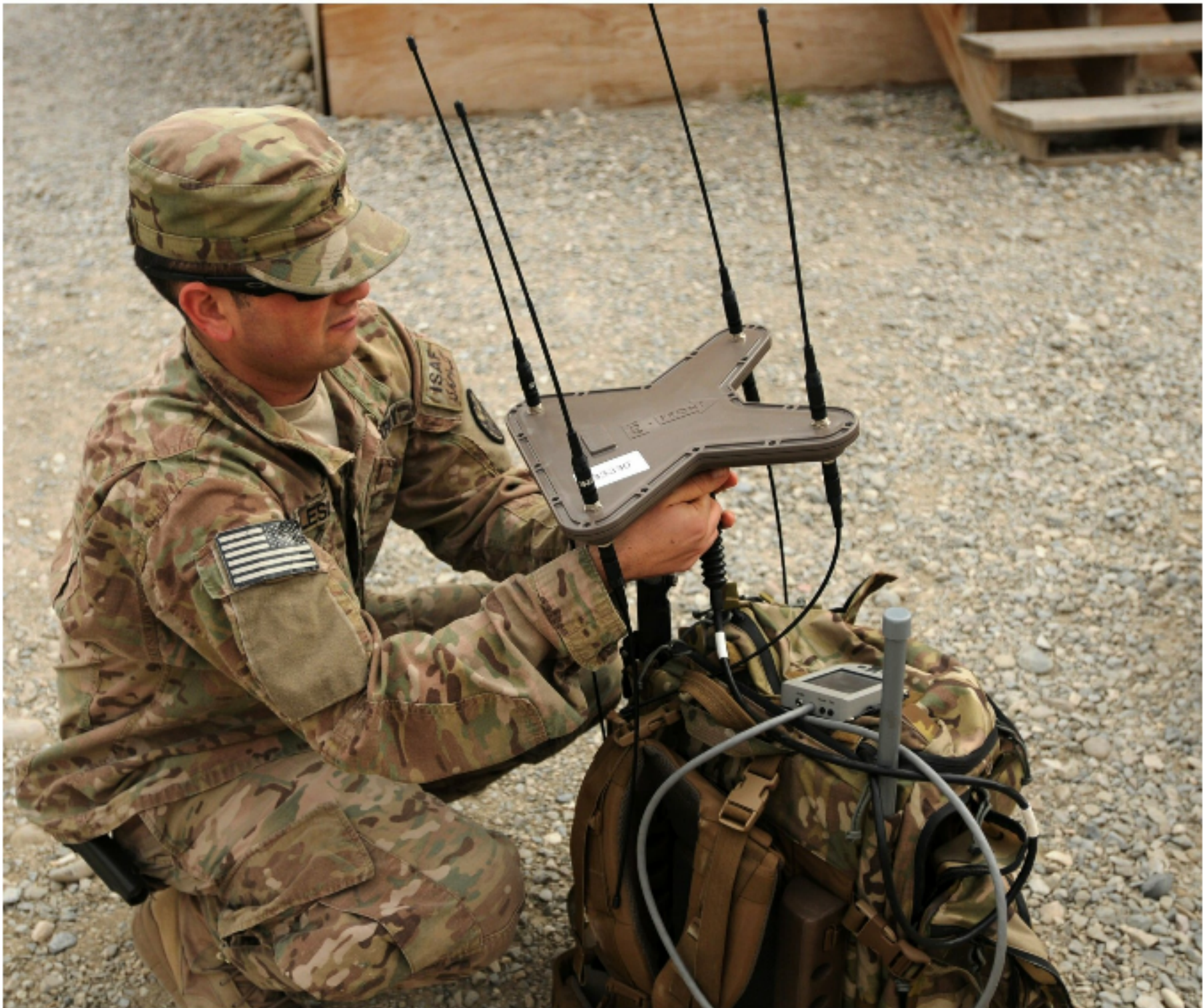
SIGINT Soldier configuring Wolfhound RDF device for targeting VHF & UHF signals.
