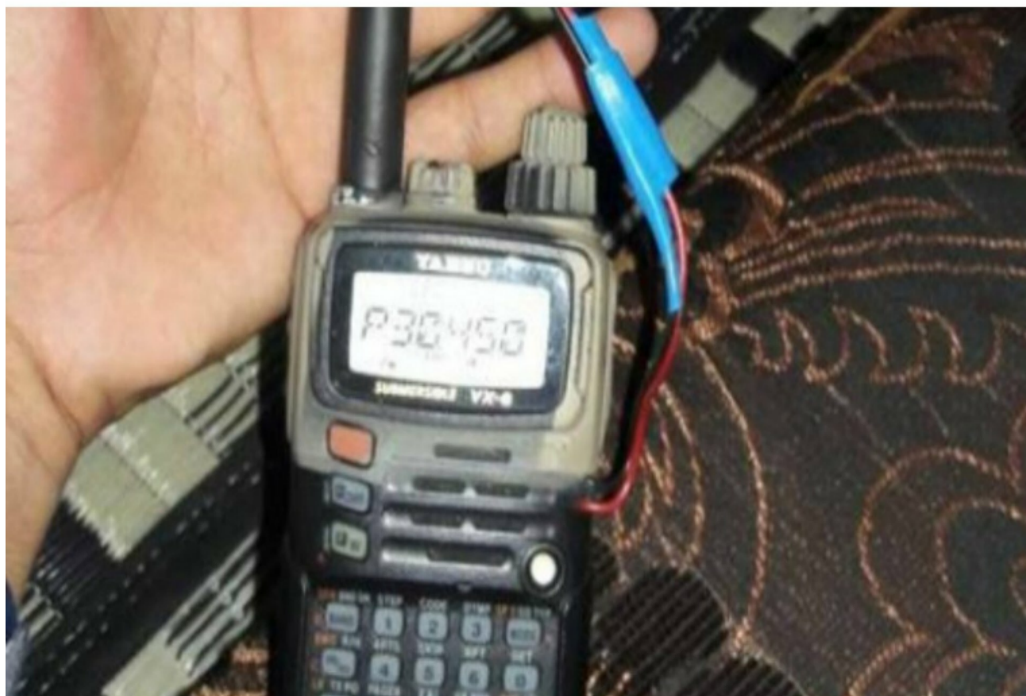
Captured ISIS Yaesu VX-6R, a multipurpose tool for communications and signals collection.
